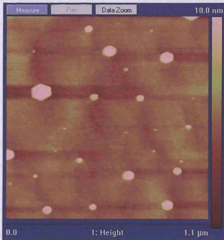
Figure 31: AFM image of Pd on TiO 2 (110) after annealing at 1000°C.
