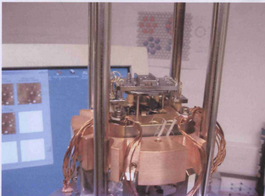
Image 4: STM head loaded with the sample and the tip. The tip is held by the scanner unit and placed over the sample
