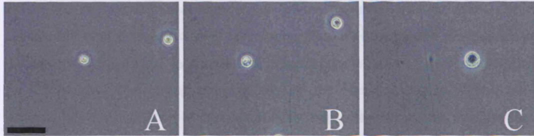
Figure 3.5: Phase contrast images of superficial (A), middle (B) and deep (C) zone articular chondrocytes immediately following isolation. Scale bar = 50µm
