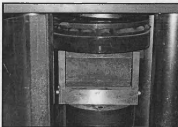
Figure 6.3: The laboratory set-up for the tensile splitting test.
