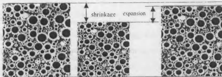
Figure 4.16: Effect of microcracking on the volume changes of hardening cement pastes. Middle: autogenous shrinkage. Right: swelling due to microcracking (Breugel, 2000).
