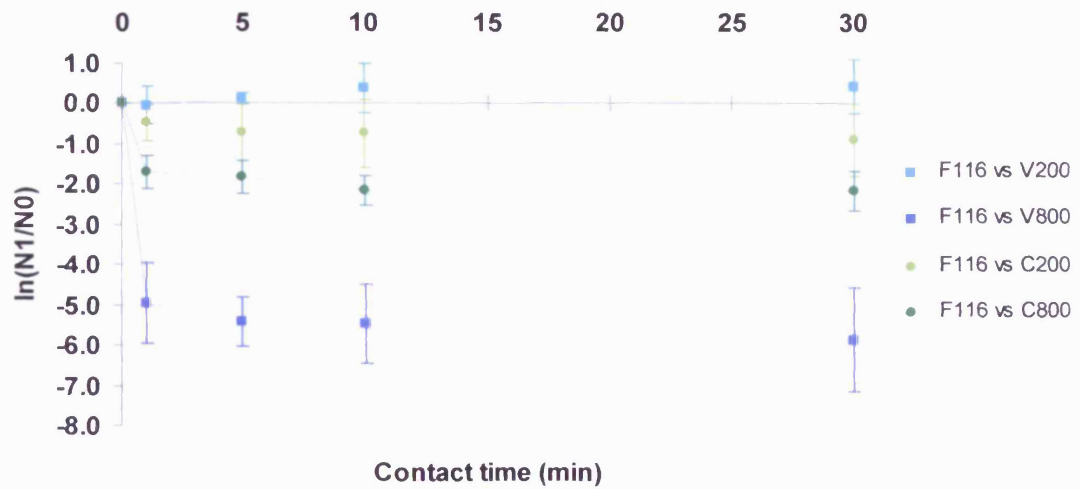
Figure 3-3. Disinfection kinetics of F116 treated with PHMB biocides at 200 and 800 ppm.
