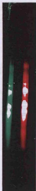
Figure 2.3: An example of a slide gel, the left lane shows Cy3 labelled cDNA and the right shows Cy5 labelled cDNA.
