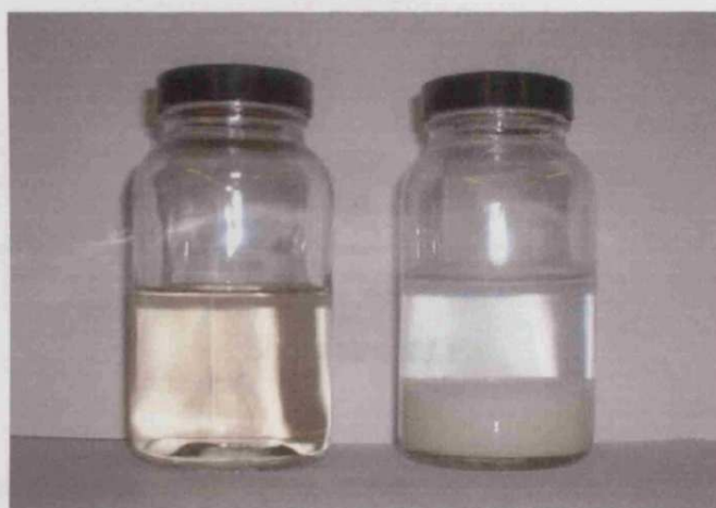
Fig 6.8(a): Joncryn 61 solution with the pH adjusted to 12 (left) using an ammonia solution and pH 4 (right) using dilute HCl. The solution without any pH adjustment is at pH 8.3 and looks identical to that of the pH 12 solution.
