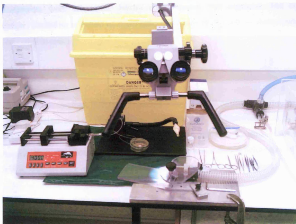
Figure 2.4 Surgical set-up used during the microinjection procedure Animals were anaesthetised in a chamber before placement on a recovery pad. Anaesthesia was maintained via an inhalation mask.
