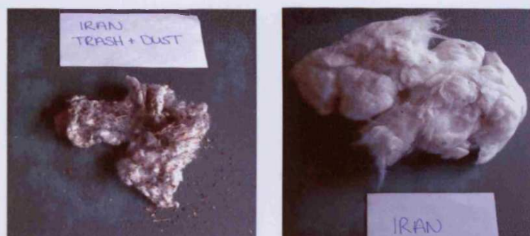
Figure 2.02: Example of trash material removed by the Shirley Analyser, compared to equivalent cotton lint sample.
