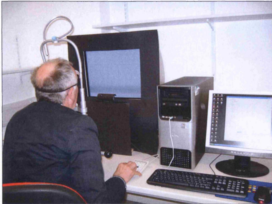
Figure 4.6 Configuration of the new hardware which comprised a high resolution cathode ray tube (CRT) monitor (Mitsubishi Diamond Pro, frame rate 70Hz, resolution 1024 x 768 pixels) and a high specification graphics board, a head support and chin rest and a separate numerical keypad. The CRT monitor is controlled by an operator using the adjacent computer (Research Machines) which has a keyboard, mouse and LCD monitor.
