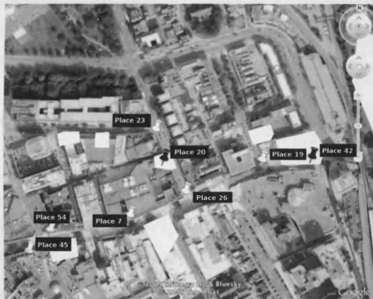
Figure 3.5: Detection of errors in urban canyons. The GPS signal was lost before reaching the destination places: Place 19, Place 23, Place 26. The places which were not correctly identified due to errors in the GPS readings are: Place 7, Place 45, Place 54.
