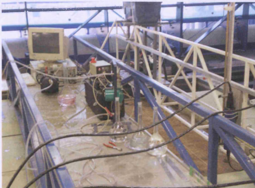
Figure 5.72: Tracer tests instrumentation: pumps, fluorometer, computer for downloading data and standard solution ready for the tests.
