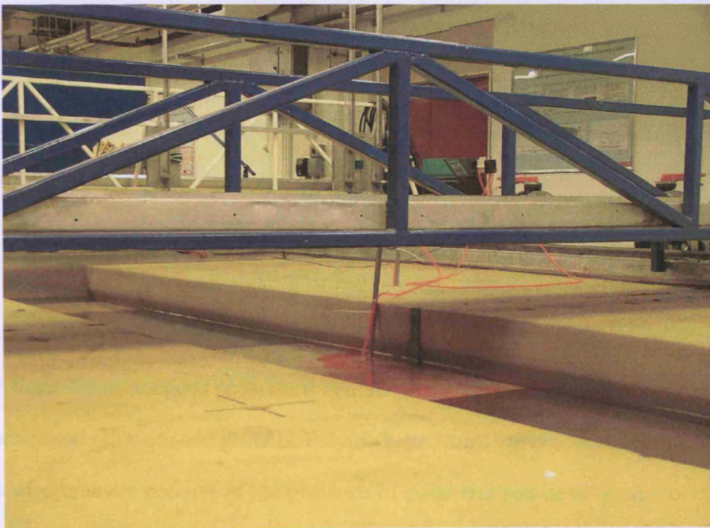
Figure 5.22: Tracer tests in the foam
