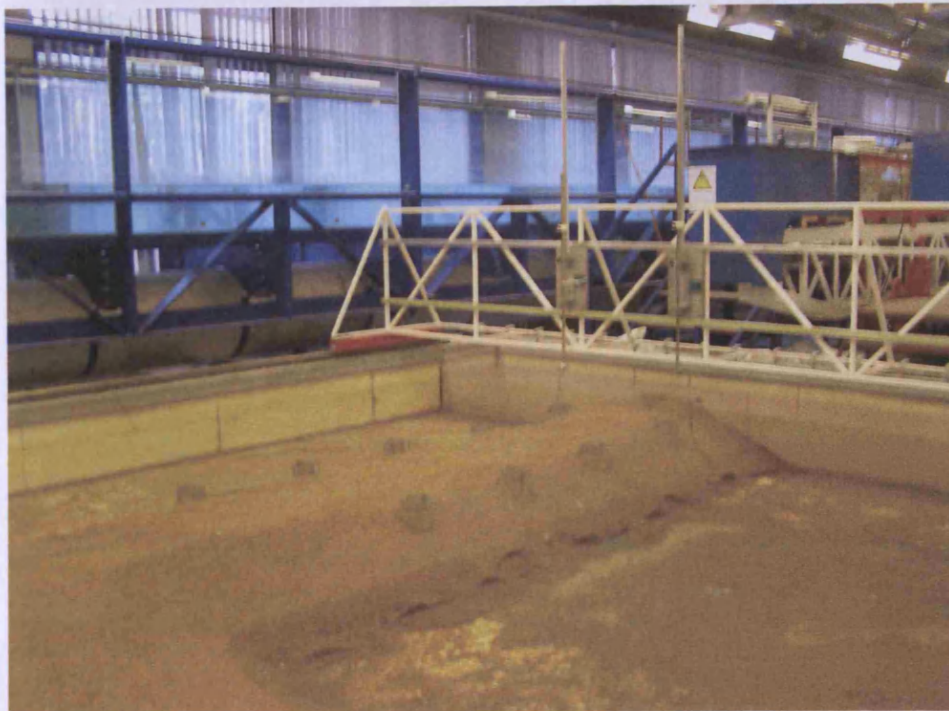
Figure 5.24: Sand embankment in the tidal basin before pumping of water
