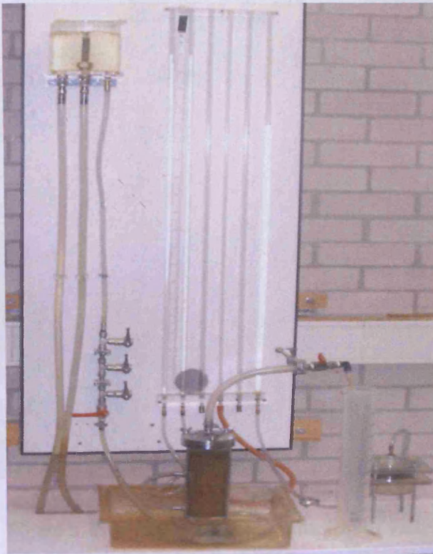
Figure 5.23: Laboratory set up for determination of hydraulic conductivity of sand
