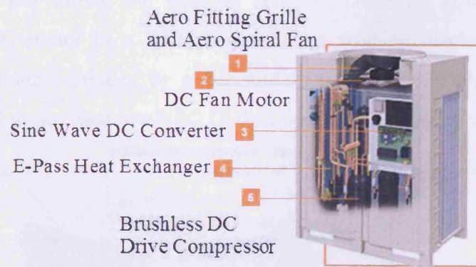
Fig. 1-11 Brushless PM DC Drive compressor with a Daikin Variable Refrigerant Volume (VRV) System [1-48]
