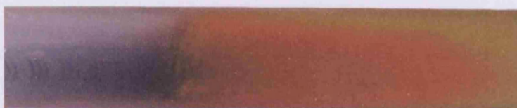
Figure 3.6: Layer experiment, showing blue-violet [\text{InBr}(\text{tmeda})] and red-purple uncoordinated \text{InBr} .
