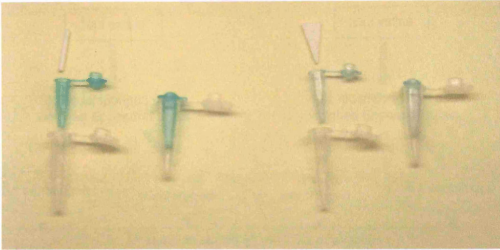
Figure 3.5 Eppendorf set up for centrifuging tear collection material
