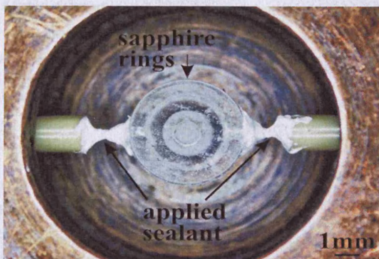
Figure 6.14. Photograph of the applied DOW CORNING ® 730 Fluorosilicone sealant on the inlet/outlet microcapillary segments of the miniaturised SDR based microfluidic device (taken with a Nikon SMZ800 electron microscope).
