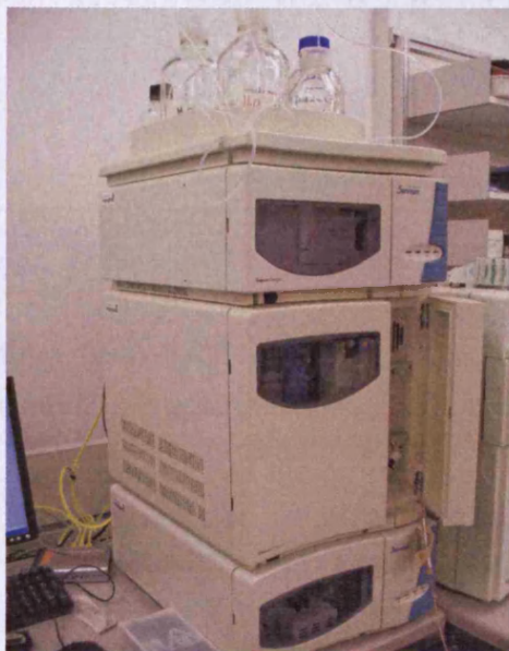
Figure 5.16. The Surveyor® LC pump is at the bottom of stack; the solvent containing vessels are on top.
