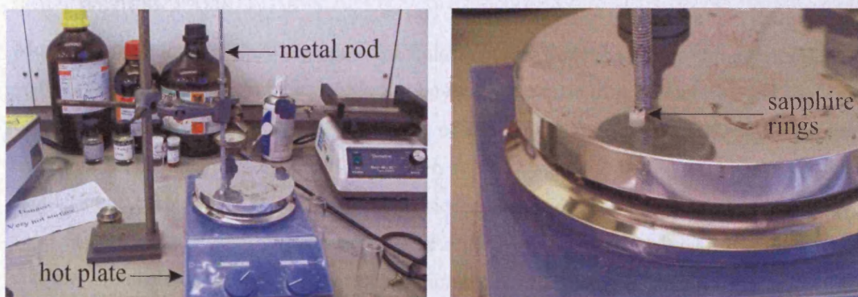
Figure 6.12. Photographs showing the setup used for bonding of the sapphire rings of miniaturised SDR.
