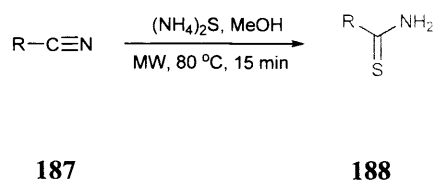
Scheme 93. Facile methods for synthesis of primary thioamides under MW irradiation at 80 °C.
