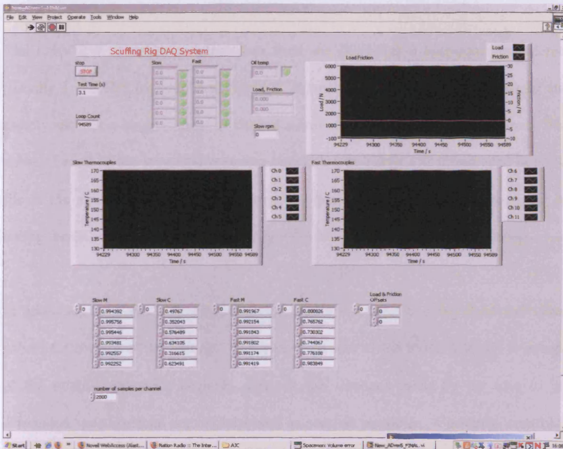
Figure 3.20: User interface (“front panel”) of the LabVIEW software for the test rig
