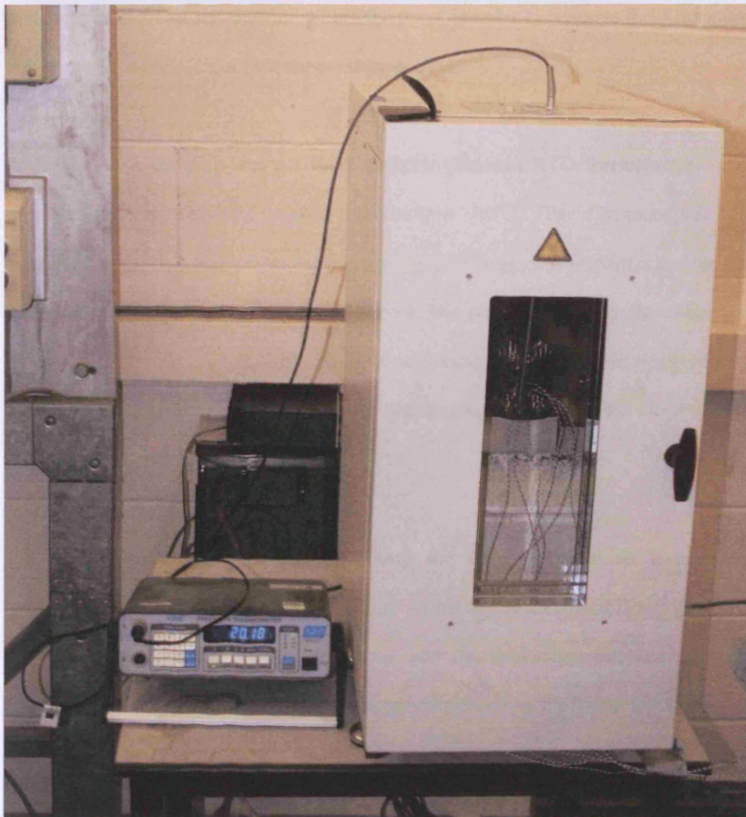
Figure 3.30: Thermocouple calibration using temperature-controlled oven and PRT
