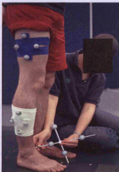
Figure 4.38 The identification of a bony landmark (medial malleolus) using the pointer. Other bony landmarks identified during the calibration include the medial and lateral epicondylar gaps and the upper border of the greater trochanter.
