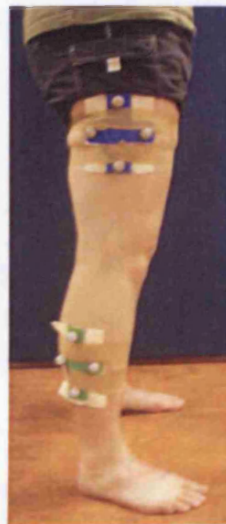
Figure 2.5 Marker clusters positioned laterally on the shank and thigh and secured using Coban™ tape
