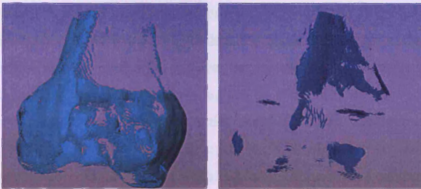
Figure 6.21 original masks created using (a) ScanIP and (b) a combination of SliceOmatic + Geomagic, minus the intersection between them.
