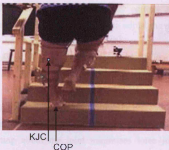
Figure 5.29 Video camera image of patient producing large adduction moment. The estimated KJC and COP are identified.
