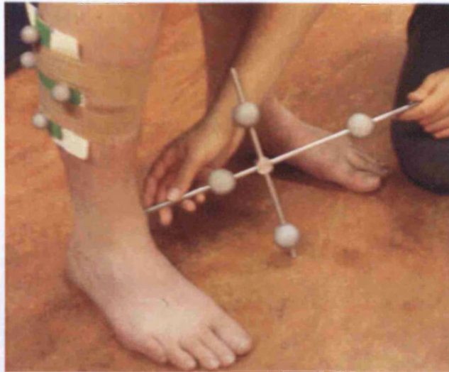
Figure 2.7 Identification of an anatomical landmark using the point of a marked aluminium pointer containing retro-reflective markers
