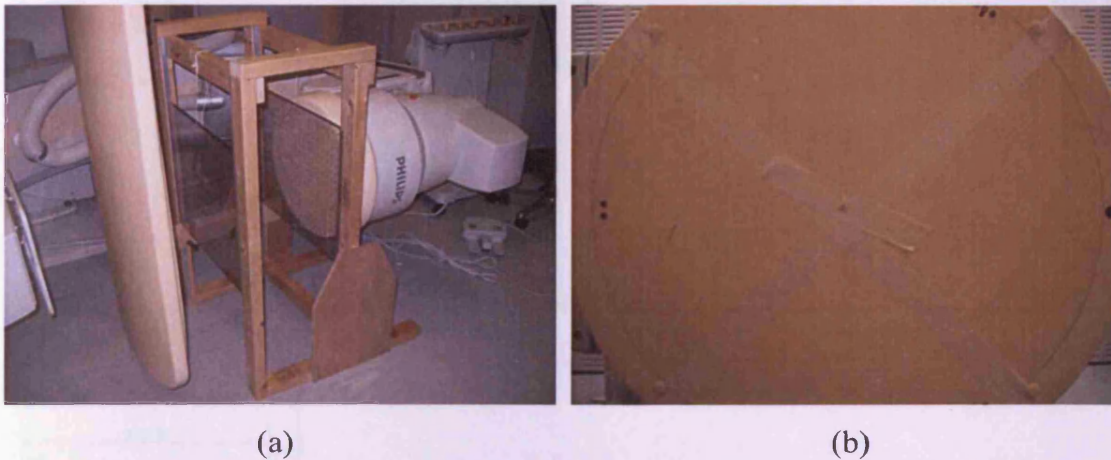
Figure 6.3 (a) C-arm position and calibration frame; (b) Defining the centre of the intensifier
