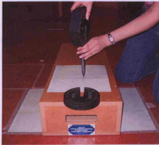
Figure 4.7 Initial method of performing accuracy tests. Step 1 is positioned on the panel on FP1. A weight is applied to a chisel pointing at a known location
