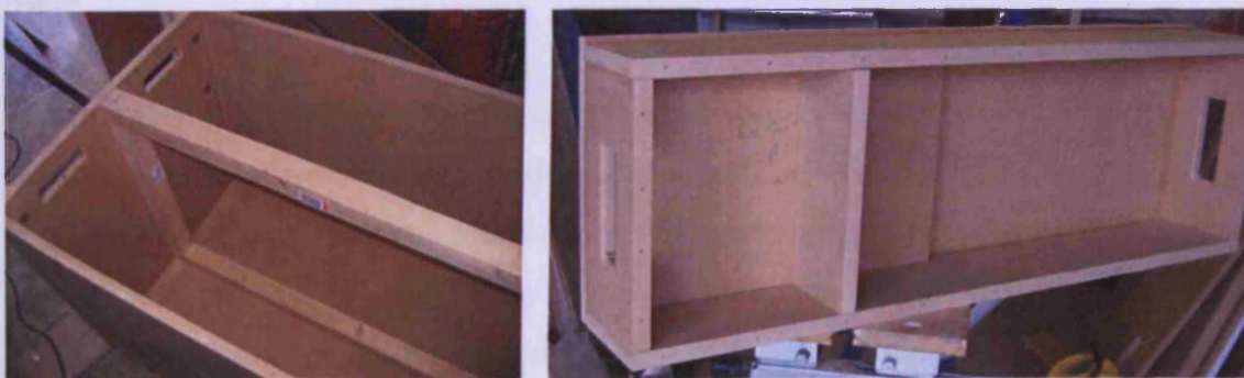
Figure 4.3 Horizontal and vertical reinforcements used to strengthen and prevent deformation.
