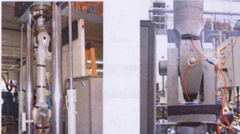
Figure 5.10: The side stay component in the test rig, showing the sensor attachment position for investigation 1
