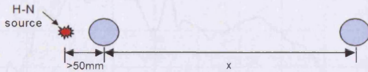
Figure 3.11: Wave velocity calculation: experimental configuration
