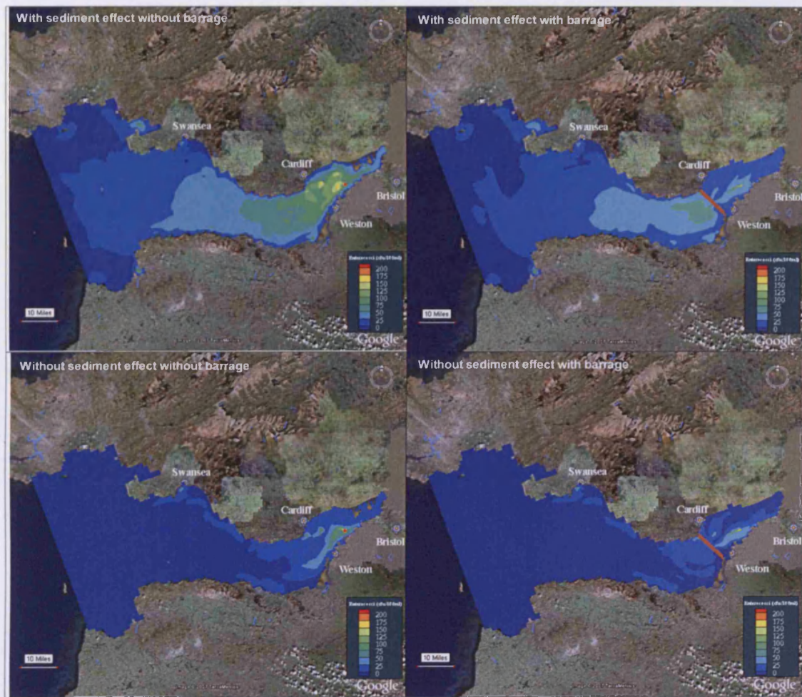
Figure 7.47 Enterococci concentrations at mean flood tide both without and with the barrage and with and without sediment-bacteria interactions
