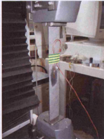
Figure 5.10. Test sample clamped at both ends having strain gauges attached at the centre of the sample.
