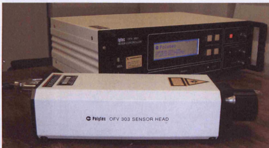
Figure 3.14. Single point laser vibrometer (Polytec GmbH) for measuring displacement caused by magnetostriction
