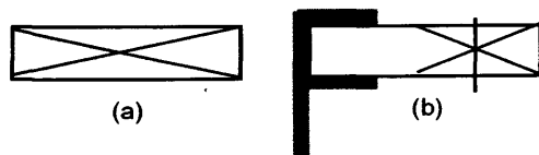
Fig. 1. Resonance condition of the sample with (a) free end and (b) clamped end
