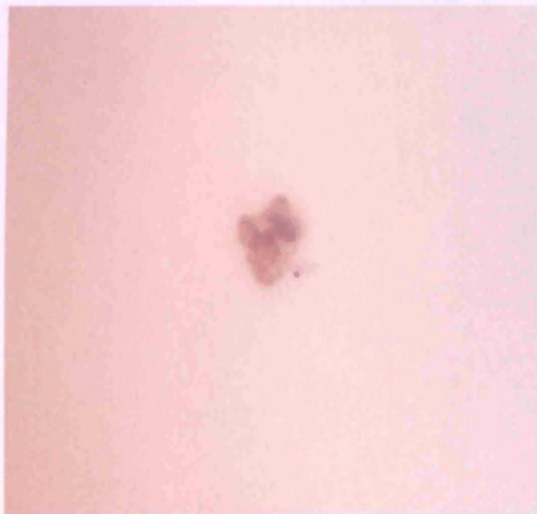
Figure 5-9. The surface of a particle of Purolite A100 taken under an optical microscope.
