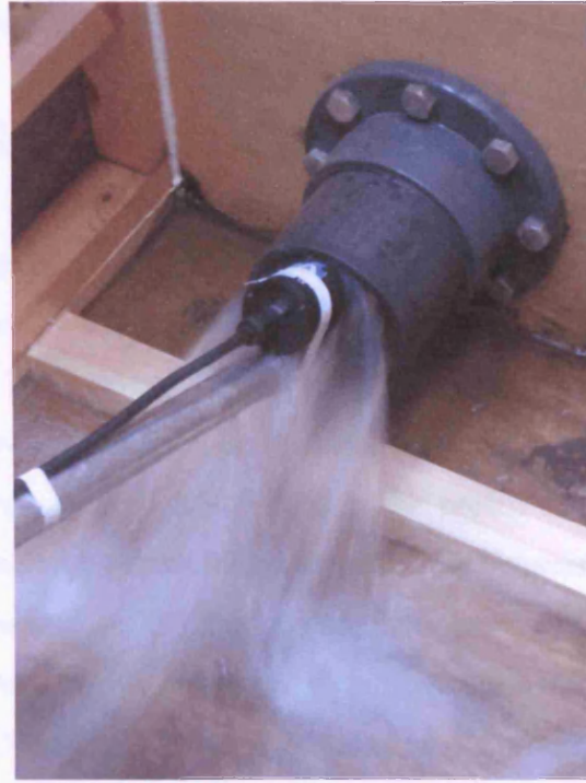
Figure 9-6. (Provided by Ian Guymer ©2004). SCUFA placed into the underflow.
