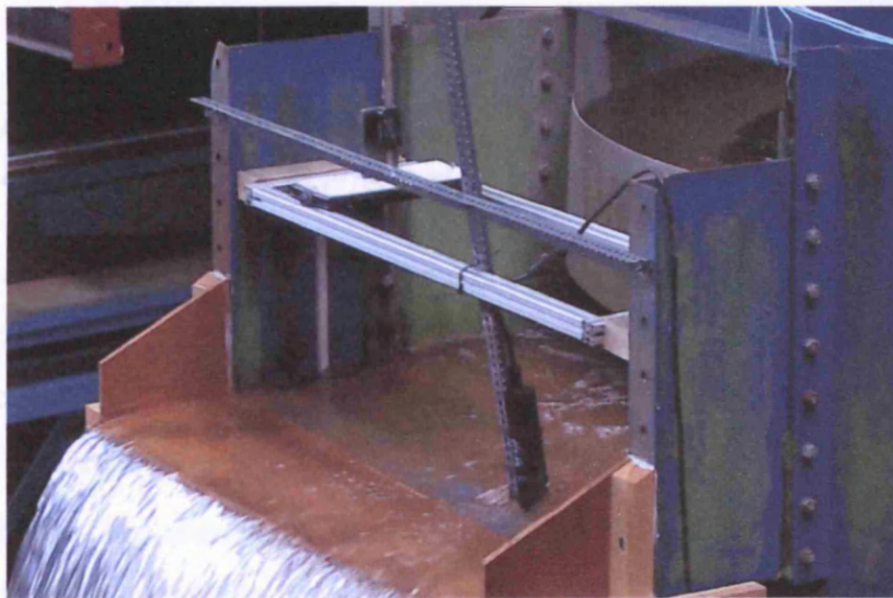
Figure 9-23. (Provided by Ian Guymer ©2004). Position of the SCUFA in the overflow.
