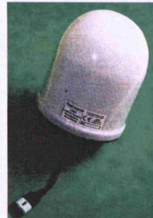
The Leafnut system's Branchnode, which controls and monitors up to 256 street lights via wireless network
