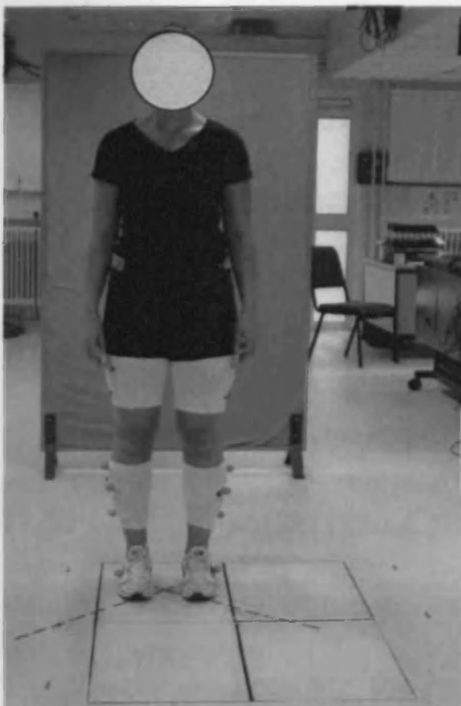
Figure 3.12: Standing balance recorded during quiet standing on a force platform
