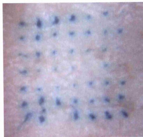
Fig. 4 Methylene blue staining of ex vivo human skin. A 49 microneedle array of 250 µm microneedle length was mounted onto the inverted syringe applicator and applied to human skin. The presence of blue staining confirms successful interruption of the stratum corneum barrier
