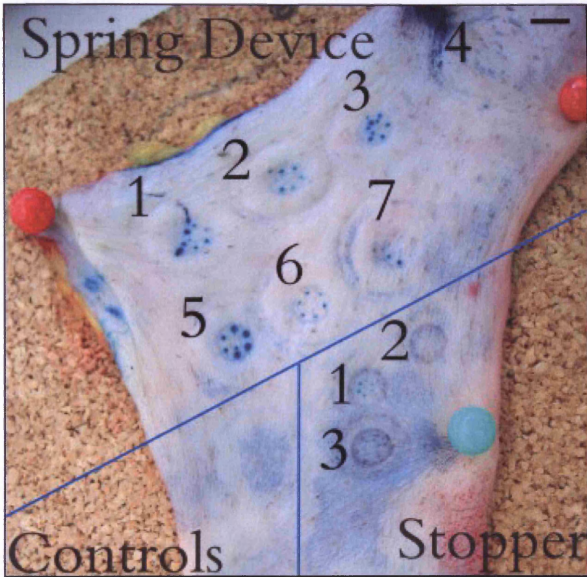
Figure 5.22. Testing of spring-loaded applicator on an ex-vivo skin sample. 1-4: applications using the spring device stained post-application, 5-7: applications using the spring device stained pre-application. 1-3 and 5-7 were applications with the cap fully raised and spring fully compressed before release on the skin surface. However, application 4 was with the spring not compressed and just pushing the device into the skin. The stopper applicator was raised to a vertical height of 5cm and then jabbed into the skin with the same researcher attempting to maintain similar pressure, force and trajectory. The controls show a larger imprint of the spring device only, with no microneedle array attached. (Bar = 5mm)
