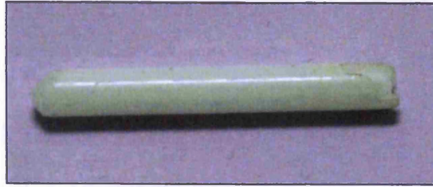
Figure 5.11. PCL rod formed from PDMS mould of a glass rod. Polycarbonate microneedle array was mounted on the end (right-hand side of photo). The rod was made to a length of 7.5cm and cut down to 5cm and 2.5cm to assess the length of leverage on microneedle puncture.
