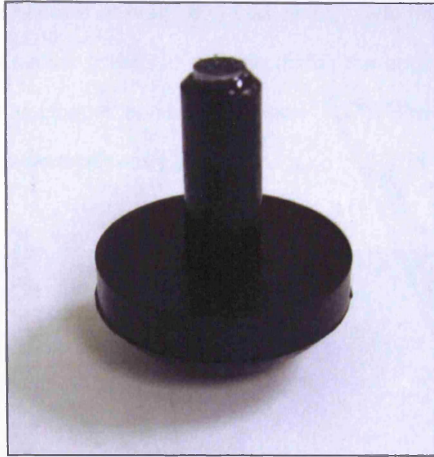
Figure 5.15. Rubber stopper used as applicator. The larger top surface provides area for grip whilst the short cylindrical stem is firm enough to not bend during rolling application. Microneedle array [B] mounted on the end.
