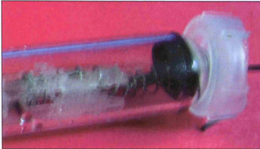
Figure 5.20. Stage 2 spring-loaded applicator. The syringe plunger has been cut to slide inside the spring, thus when the plastic cap (right) is pulled back, the spring coils over the plunger and compresses straight. The black rubber stopper was needed to prevent this spring from popping out of the hole at the round-bottom end of the Falcon tube. This spring-loaded applicator with microneedle array mounted on the end was used to apply the microneedles into the skin from a vertical position perpendicular to the skin.
