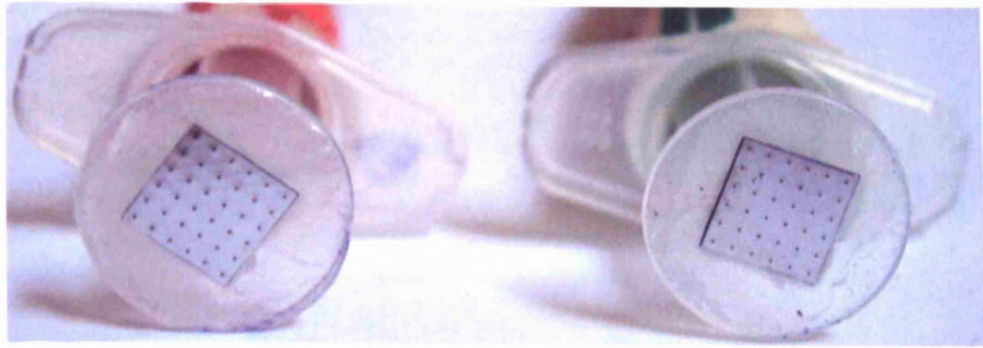
Fig. 5 Microneedle arrays of 180 and 280 \mu\text{m} length mounted onto inverted syringe applicators
