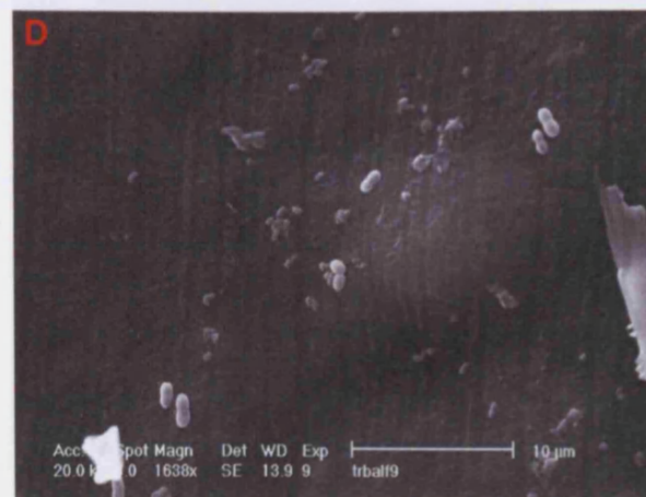
Figure 36: Scanning electron micrographs of an all-silicone catheter inflated with 10 mg/ml triclosan in 5% PEG that drained freely in the model for 7 days and was fixed without RHT. These images are taken of the catheter eye-hole and at intervals down the length of the catheter. Image A reveals little sign of catheter encrustation, but highlights the surface irregularities resulting from engineering techniques used to create the eye-hole. Only very small groups of bacteria were visible, many of which appeared smaller than on the control catheter, and often appeared to be deformed.
