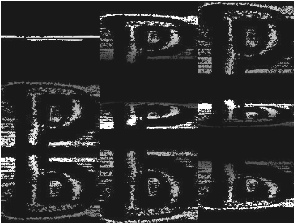
Figure 2-4: An OCT tomogram montage of a coin acquired with the FFSSOCT system. This image was composed of 512 interference images, acquired in 5.2 seconds and has lateral dimensions of 640x480 pixels (970x730 \mu m) and an axial dimension of 128 pixels (260 \mu m). The projection of the volumetric image has been rotated in 40 degree steps, starting from the top left and finishing in the bottom right.
