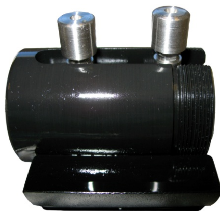
Figure 2.16. The sample chamber designed for spectrophotometry study.
