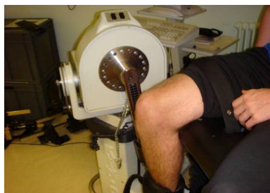
(Figure 4.3.4.1.b) Knee position to the centre of rotation to the centre lever arm
