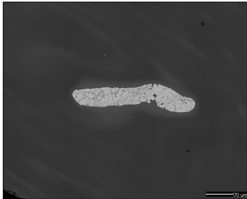
Figure 5.1.46 – BSE micrograph showing ‘dark’ sample ERL104:G144:2559, a Dark Globular bead. A fragment of iron scale (pale grey) is visible in a soda-lime-silica glass matrix (dark grey).
