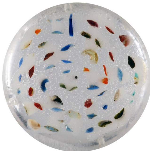
Figure 2.3.3 – A photograph showing a polished sample block containing glass samples from Eriswell. Note the larger dark blue glass standard (Corning A) at the top of the image, which is orientated so as to provide a ‘north point’. Resin block is approximately 3cm in diameter.
