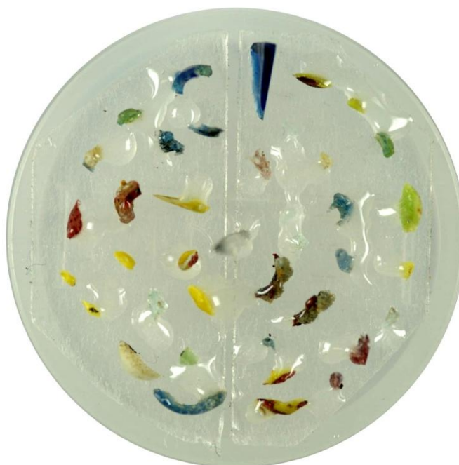
Figure 2.3.2 – A photograph showing glass samples from Eriswell mounted on a 3cm resin block mould base using double-sided tape and Araldite™ 5-minute epoxy resin. Note the larger dark blue glass standard (Corning A) at the top of the image, which is orientated so as to provide a ‘north point’.
