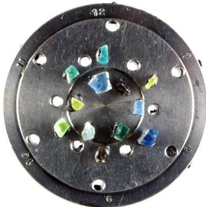
Figure 2.2.7 – A photograph showing fragments of Early Byzantine glass tesserae from Caesarea, Israel, mounted on the SEM stage (approximately 6cm in diameter) for analysis by environmental scanning electron microscopy (ESEM-EDS).
