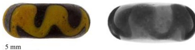
Figure 3.2.1 – Bead ERL104:G305:1871, a Melon Associated bead, showing an opaque yellow circumferential zigzag trail on a ‘dark’ bead body (left) and a positive x-radiograph of the bead (right). The opaque yellow glass appears darker in the image as it is denser, due to a much higher lead content.
