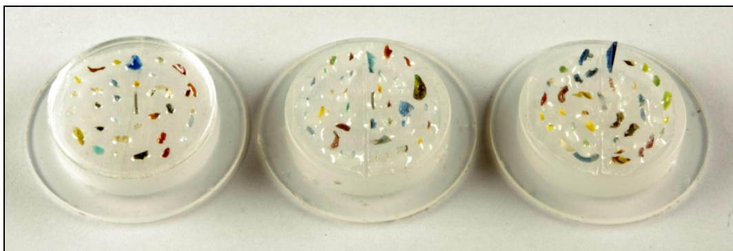
Figure 2.3.1 – A photograph showing glass samples from Eriswell mounted on 3cm resin block mould bases using double-sided tape and Araldite™ 5-minute epoxy resin.
