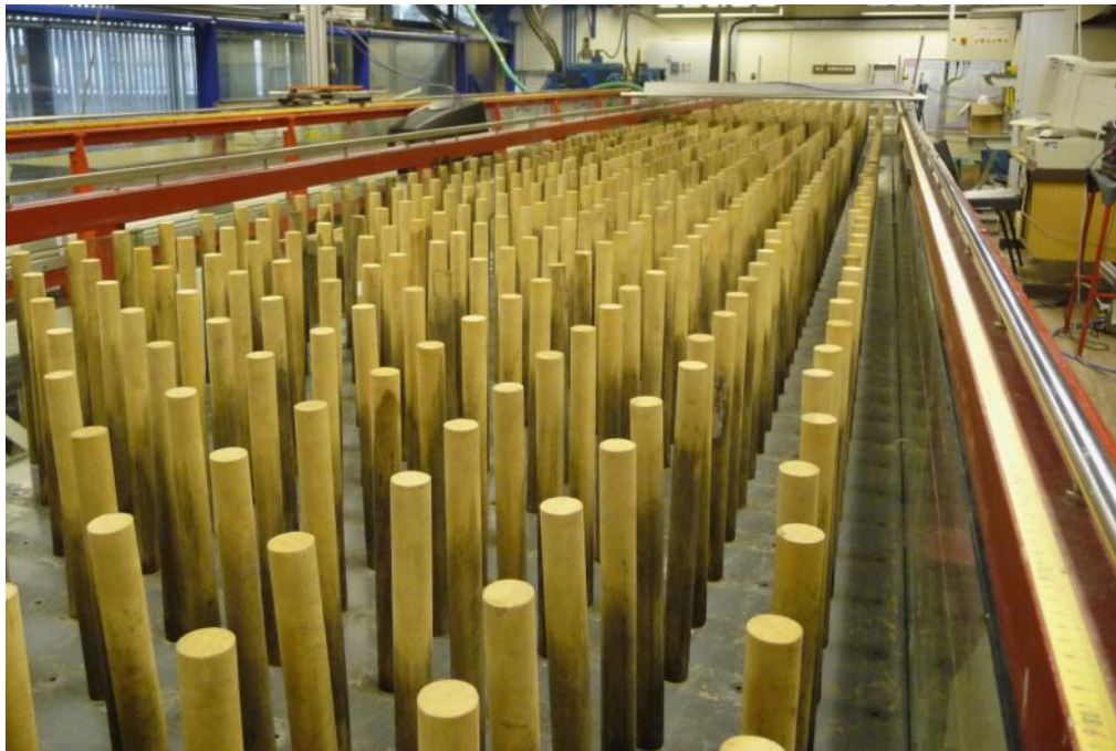
Figure 3.5 (a) Rods in aligned arrangement for test 3.90A
