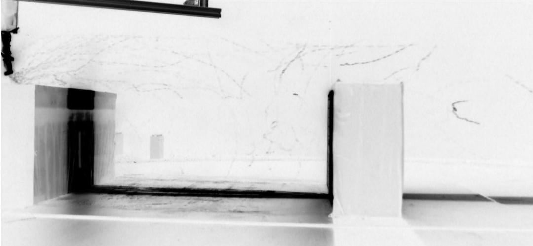
Figure 6-55: Sequence of airflow visualization by using helium bubbles in the wind tunnel (90°; H/W=0.50).
