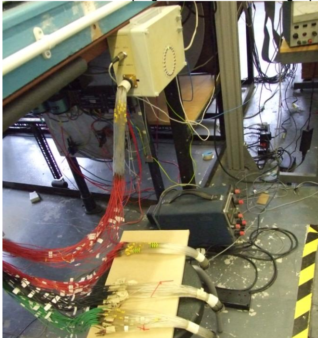
Figure 5-35: The WSA transducer and plugs used for measuring C_p 's in the WT.
