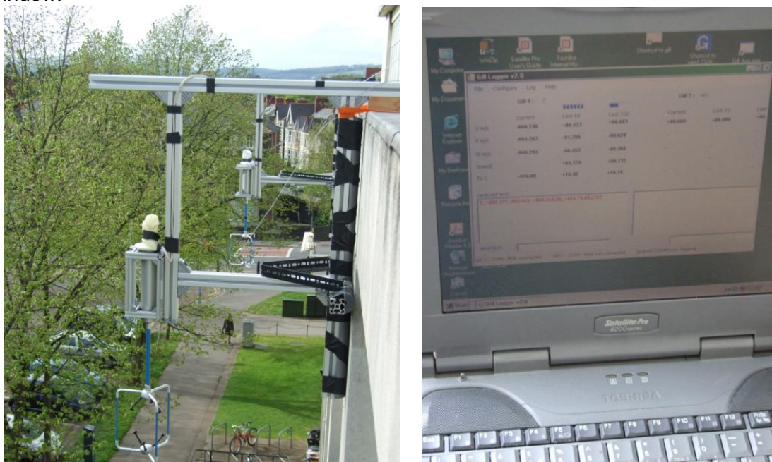
Figure 5-74: Ultrasonic anemometer probe and laptop with the data logger software window.
