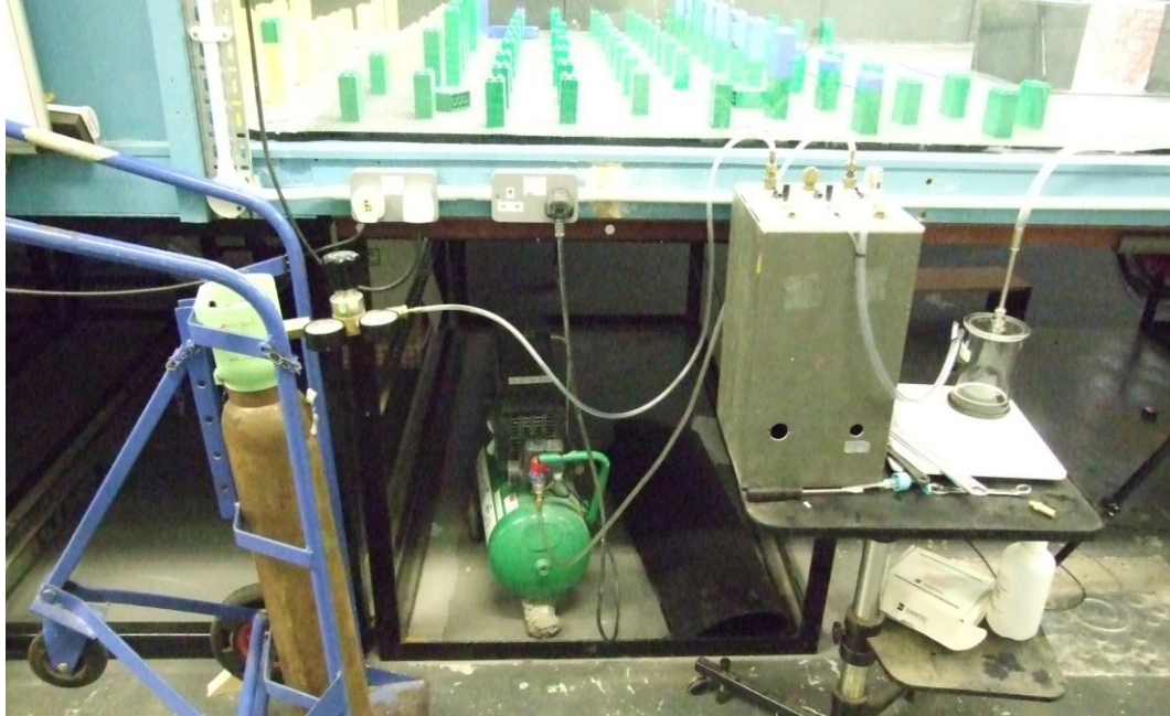
Figure 5-36: The WSA bubble generator and air compressor for airflow visualization.
