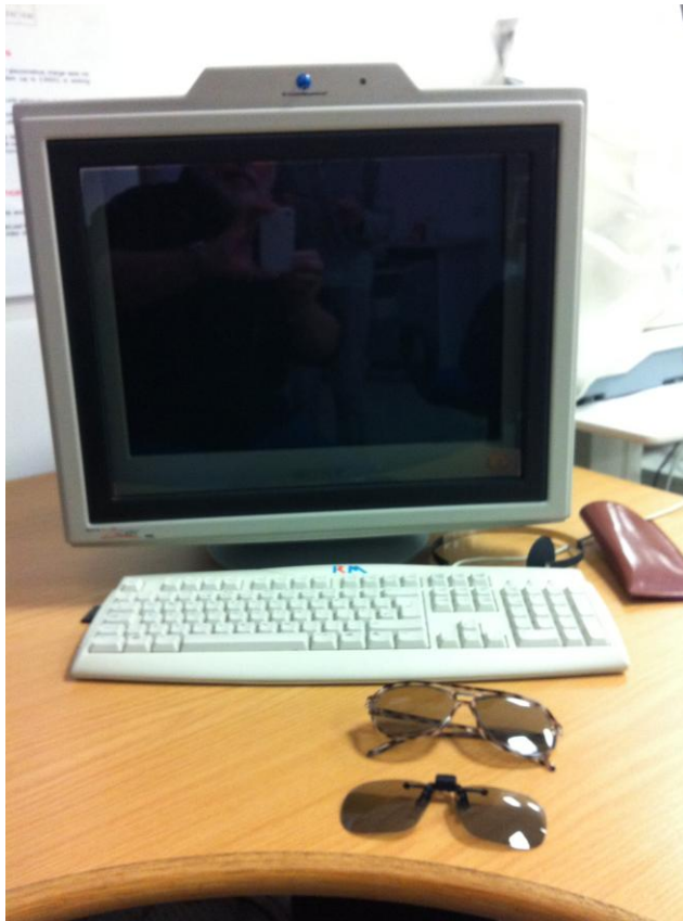
Figure 3.2. Z –screen mounted on computer monitor, with examples of passive polarised spectacles (Stereographics Corporation, CA, USA)
