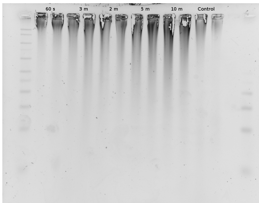
Figure 4.12: Example of alkaline gel run with vapourised hydrogen peroxide treated samples.
