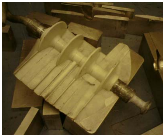
Cured weather shed housing before trimming the silicone excess
