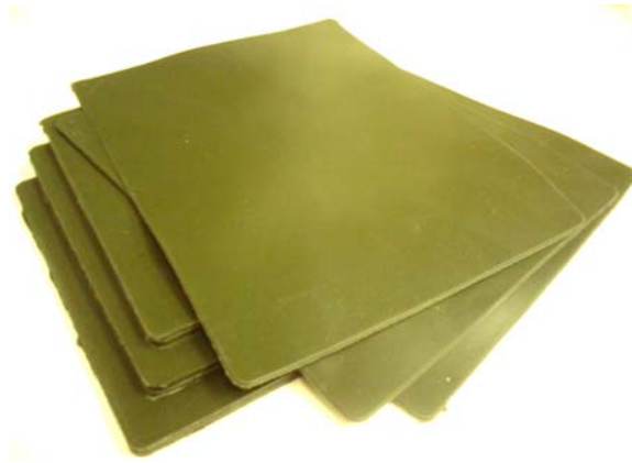
Figure 6.1: Microvaristor grading sheets supplied by manufacturer
