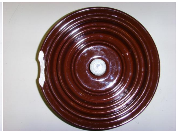
e) Bottom view – Chipped Insulator
