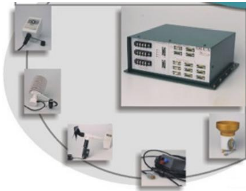
Figure 2.8: Showing OLCA acquisition and processing unit, leakage current and weather sensors. Reproduced from [27].
