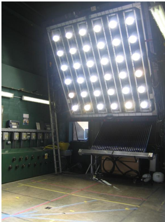
Figure 4.25: Halogen-tube array solar test facility at Cardiff University.
