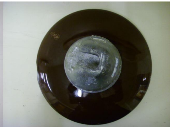
d) Top view – Chipped Insulator
