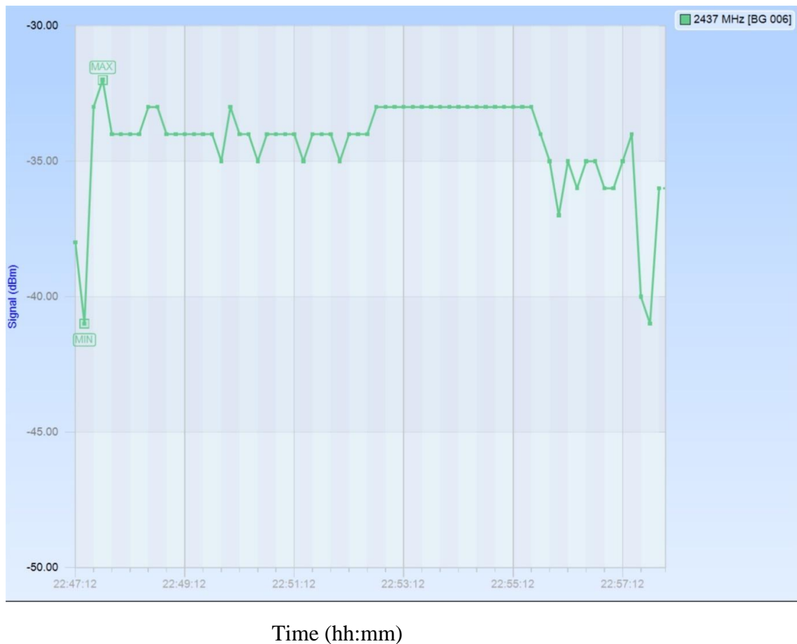
Figure C.17: Signal strength of DI-524 access point measured at WLAN Sensor - Healthy porcelain insulator fog chamber test - High voltage laboratory
