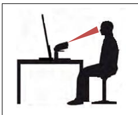
Figure 7.6 Optimum setup for the Tobii X120 eye tracker (Tobii Studio™ 2.2 User Manual 2010).
