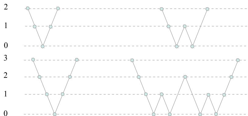
Figure 3.4. Grid levels for the V and W cycles for 2 and 3 levels (after Knabner and Angermann 2003)
