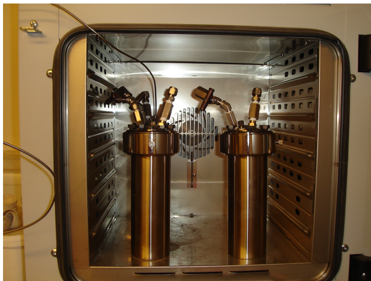
Figure 3.9 Two of the pressure vessels used for MEA degradation
