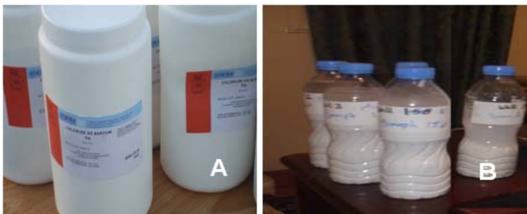
Figure 4.7 Barium chloride (A) to be add to form the CITD precipitate (B)
