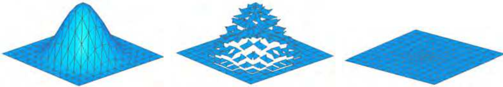
Figure 4: Base surface reconstruction. For the input mesh (left), each triangle is locally reoriented to agree with the smoothed normal field. The triangles become disconnected (center). The Poisson equation stitches the triangles together again in new positions, giving the base surface underlying the bumpyplane (right).
