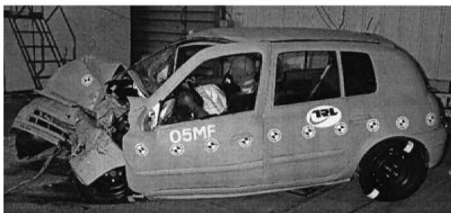
Fig. 15 Deformation for two 80 km/h ODB tests with a super-mini-sized car showing good repeatability
