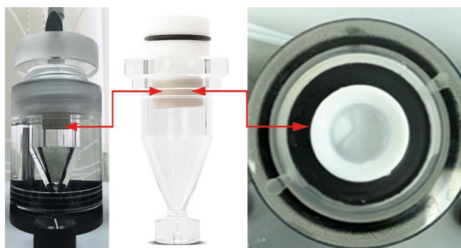
Figure 5. Flow-through cell made by ERWEKA (Germany) for oral dosage forms with adaptor for release evaluation of ointments, creams and gels
