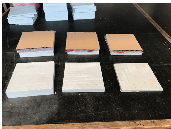
FIGURE 2 Samples tested (top to bottom, from left to right—composite 20-mm ABS, 10-mm ABS, 5-mm ABS, uniform 20-mm ABS, 10-mm ABS, 5-mm ABS)
