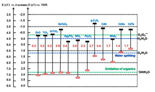
**Figure 4.** Bandgap and band edge potentials for different semiconductors. (Reproduced with permission from [37]: Kumar, S.; Karthikeyan, S.; Lee, A. g-C<sub>3</sub>N<sub>4</sub>-Based Nanomaterials for Visible Light-Driven Photocatalysis. *Catalysts* **2018**, *8*, 74, doi:10.3390/catal8020074. Copyright (2018), MDPI (Basel, Switzerland)).
