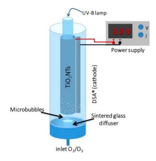
**Figure 10.** Schematic representation of the PEC annular bubble column reactor. (Reproduced with permission from [47]: Kim, J.Y.U.; Bessegato, G.G.; de Souza, B.C.; da Silva, J.J.; Zanoni, M.V.B. Efficient treatment of swimming pool water by photoelectrocatalytic ozonation: Inactivation of *Candida parapsilosis* and mineralization of Benzophenone-3 and urea. *Chem. Eng. J.* **2019**, 378, 122094; DOI:10.1016/j.cej.2019.122094. Copyright (2019), Elsevier (Amsterdam, The Netherlands)).
