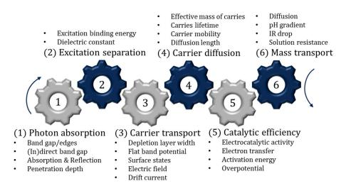
Figure 5. Sequential steps associated with photocatalysis and PECs.
