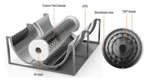
**Figure 13.** PEC reactor configuration with CPC. (Reproduced with permission from [67]: McMichael, S.; Waso, M.; Reyneke, B.; Khan, W.; Byrne, J.A.; Fernandez-Ibanez, P. Electrochemically assisted photocatalysis for the disinfection of rainwater under solar irradiation. *Appl. Catal. B* **2021**, *281*, 119485, doi:10.1016/j.apcatb.2020.119485. Copyright (2021), Elsevier Elsevier (Amsterdam, The Netherlands)).
