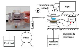
**Figure 21.** Experimental set-up, insert photo of the reactor. (Adapted with permission from [89]: Wang, X.; Wang, G.; Chen, S.; Fan, X.; Quan, X.; Yu, H. Integration of membrane filtration and photoelectrocatalysis on g-C<sub>3</sub>N<sub>4</sub>/CNTs/Al<sub>2</sub>O<sub>3</sub> membrane with visible-light response for enhanced water treatment. *J. Membr. Sci.* **2017**, *541*, 153–161, doi:10.1016/j.memsci.2017.06.046. Copyright (2017), Elsevier (Amsterdam, The Netherlands)).
