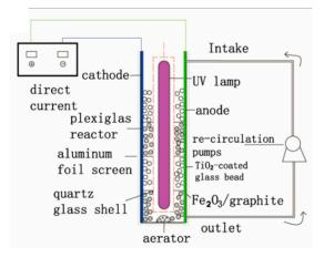
**Figure 26.** Schematic diagram of the three-dimensional electrode packed bed photocatalytic reactor. (Reproduced with permission from [106]: Liu, R.; Zhang, Y. Highly efficient degradation of berberine chloride form wastewater by a novel three-dimensional electrode photoelectrocatalytic system. *Environ. Sci. Pollut. Res.* **2018**, *25*, 9873–9886, doi:10.1007/s11356-018-1293-y. Copyright (2018), Springer Nature (Heidelberg, Germany)).
