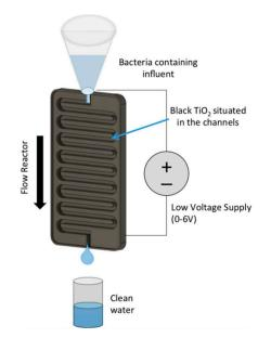
**Figure 16.** Schematic of a channel reactor using titanium nanotubes annealed in 2% hydrogen. (Reproduced with permission from [70]: Carlson, K.; Elliott, C.; Walker, S.; Misra, M.; Mohanty, S. An effective, point-of-usewater disinfection device using immobilized black TiO<sub>2</sub> nanotubes as an electrocatalyst. *J. Electrochem. Soc.* **2016**, *163*, H395–H401, doi:10.1149/2.0651606jes. Copyright (2016), IOP Publishing (Bristol, UK)).
