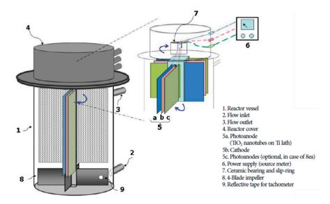
**Figure 18.** Rotational reactor using titanium nanotube photoanode and titanium cathode. (Adapted with permission from [78]: Cho, H.; Seo, H.S.; Joo, H.; Kim, J; Yoon, J. Performance evaluation of rotating photoelectrocatalytic reactor for enhanced degradation of methylene blue. *Korean J. Chem. Eng.* **2017**, *34*, 2780–2786, doi:10.1007/s11814-017-0198-7. Copyright (2017), Springer Nature (Seoul, Korea)).
