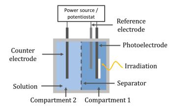
Figure 23. Two-compartment reactor set-up.
