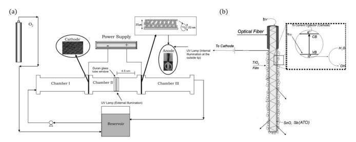
**Figure 20.** (a) Schematic representation of the experimental set-up, (b) fibre optic photoanode. (Adapted with permission from [85]: Esquivel, K.; Arriaga, L.G.; Rodríguez, F.J.; Martínez, L.; Godínez, L.A. Development of a TiO<sub>2</sub> modified optical fiber electrode and its incorporation into a photoelectrochemical reactor for wastewater treatment. *Water Res.* **2009**, *43*, 3593–3603, doi:10.1016/j.watres.2009.05.035. Copyright (2009), Elsevier (Amsterdam, The Netherlands)).
