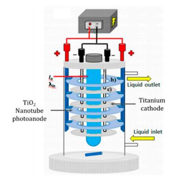
**Figure 11.** Schematic representation of the experimental set-up using anodised titanium photoanode. (Adapted with permission from [63]: Montenegro-Ayo, R.; Morales-Gomero, J.C.; Alarcon, H.; Cotillas, S.; Westerhoff, P.; Garcia-Segura, S. Scaling up Photoelectrocatalytic Reactors: A TiO<sub>2</sub> Nanotube-Coated Disc Compound Reactor Effectively Degrades Acetaminophen. *Water* **2019**, *11*, 2522, doi:10.3390/w11122522. Copyright (2019), MDPI (Basel, Switzerland)).
