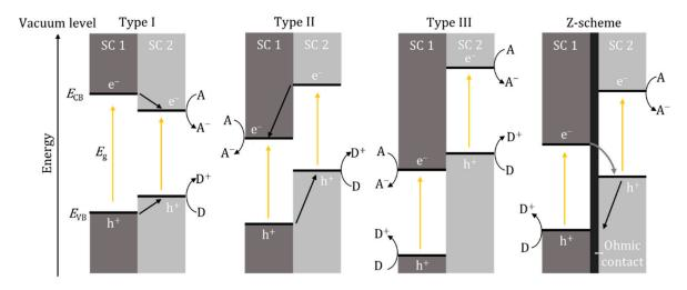
**Figure 6.** Band edge positions and electron/hole movement for type I, II and III heterostructures and z-scheme. SC—semiconductor, A—electron acceptor, D—electron donor, e<sup>-</sup>—electron, h<sup>+</sup>—hole.
