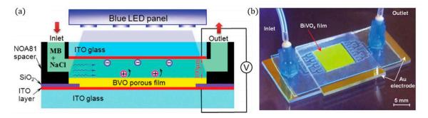
**Figure 17.** (a) Cross-sectional view of the reaction chamber, (b) photo of the PEC microreactor. (Adapted with permission from [49]: Wang, N.; Zhang, X.; Chen, B.; Song, W.; Chan, N.Y.; Chan, H.L.W. Microfluidic photoelectrocatalytic reactors for water purification with an integrated visible-light source. *Lab Chip* **2012**, *12*, 3983–3990, doi:10.1039/c2lc40428a. Copyright (2012), Royal Society of Chemistry Publishing (Cambridge, UK)).
