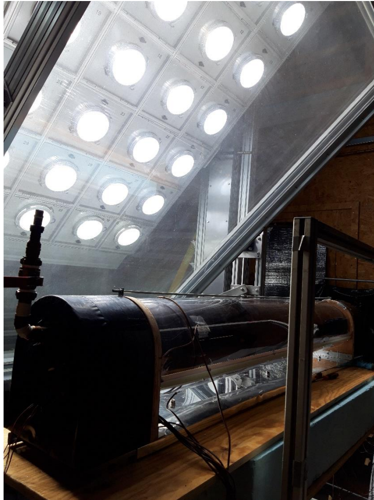
Figure 4: Typical experimental set up for a prototype under the solar simulator
