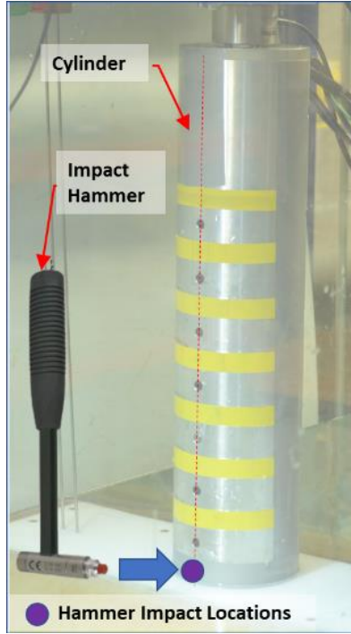
Figure 14 Impact hammer tests and impact location
