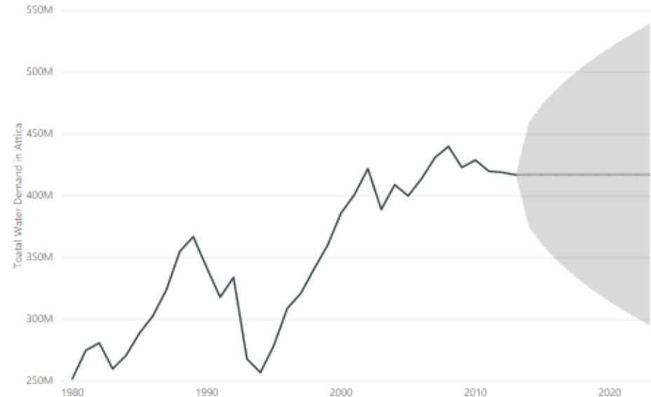
Figure 2: Annual water demand in the research area and 10-year ahead estimation with prediction intervals
