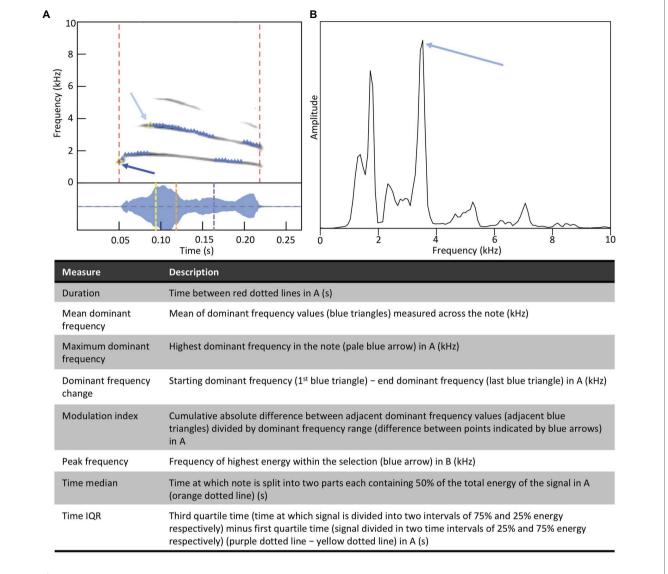
FIGURE 5 | Definitions of acoustic characteristics measured for each note. Panels A and B support definitions presented in the table.
