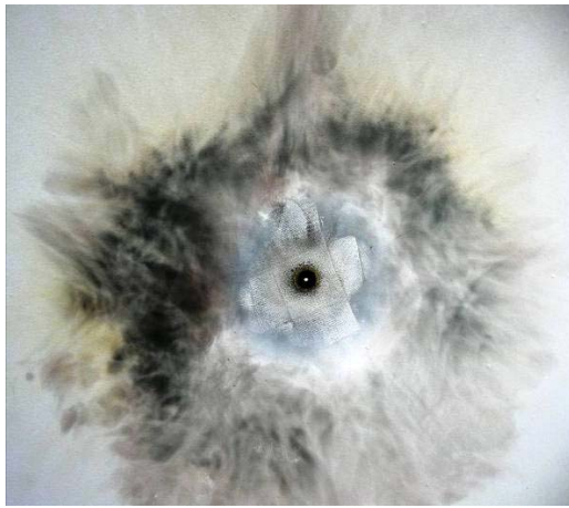
Fig. 12. General view from the binding zone on the outer surface of the TS of a flat duralumin panel ( h=1.5 mm) of the airplane's fuel tank of the plasma channel simulated at the UITOM-1 type installation of the lightning discharge of the results of the direct impact on this TS for zone 1A of the normalized components of the artificial lightning current, characterized by local thermal damage of the wall of the TS of the panel at the place of impact of the lightning channel to it
