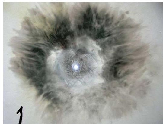
Fig. 16. General view from the binding zone on the outer surface of the TS of a flat duralumin panel ( h=1.2 mm) of the aircraft's fuel tank of the plasma channel simulated by the UITOM-1 installation of a lightning discharge of the results of direct exposure to this TS for zone 1A of the normalized components of the artificial lightning current, characterized by through penetration of the TS panel wall at the point of impact of the lightning channel
