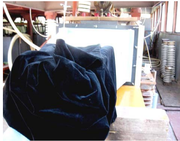
Fig. 7. Appearance of a pyramidal LTC with a camera at its small end (the camera is covered with a black lightproof protective cover) during the current registration of thermal sparks from the internal surface of the TS, rigidly and vertically mounted on its large end
