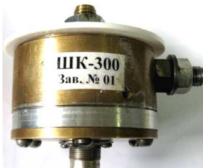
Fig. 4. General view of a measuring disk shunt of a coaxial design of the ShK-300M1 type, installed in a high-current discharge circuit of a high-voltage test setup of the UITOM-1 type and used for simultaneous recording on the screens of three storage oscilloscopes of ATPs of A (D)-, B- and C (C*)- components of the artificial lightning current [17, 18]
